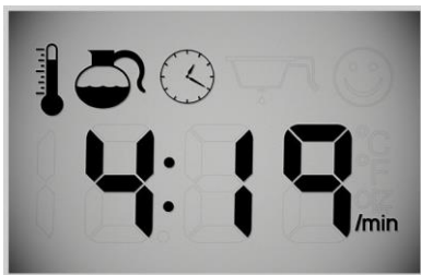
Close-up of TVT display Time/Temp/Volume
